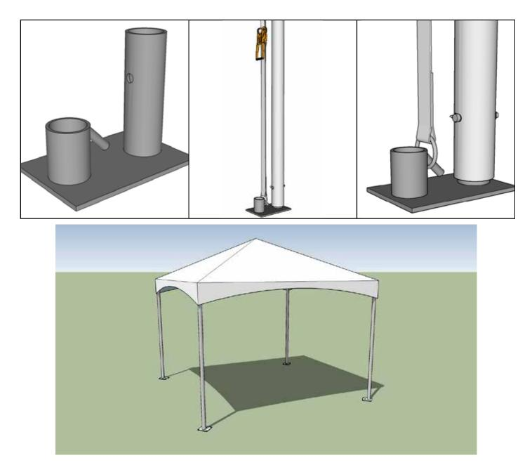
8. At each leg, now drive a tent stake into the ground about 5' from the edge of the tent. Attach the Guy Ropes provided with your tents and tighten securely to the tent stake. provided. In the event of high winds, the cover should be removed from the frame to prevent damage to your tent. Your tent should be vacated during inclement weather.
